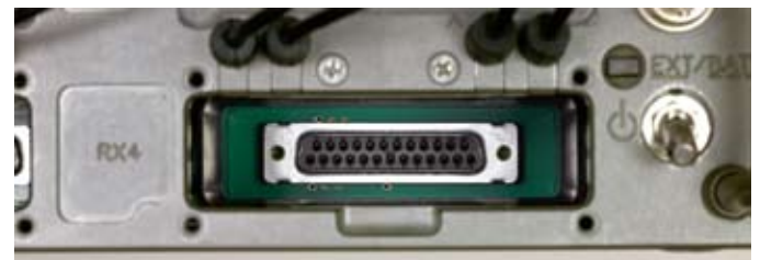
Receivers interface with the Octopack board via a 25-pin connector and the Unislot adapter.
