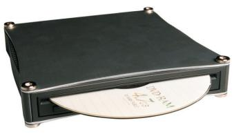
The XL-DVDRAM is an external FireWire (-1394a) optical drive for use with Sound Devices 7-Series Digital Recorders. Based on the Panasonic UJ-85 Multi-drive mechanism (5X DVD-RAM) the XL-DVDRAM drive becomes an available storage volume for either direct recording or file copying to a 7-Series recorder. The XL-DVDRAM is bus-powered directly from the FireWire port of the 7-Series recorder. No additional power source is required.
